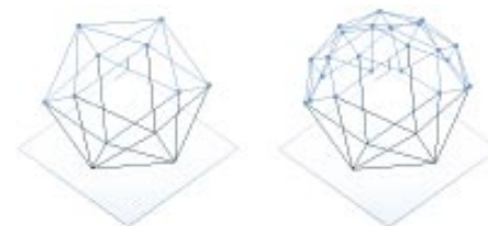
An object with added vertices using the Subdivide command.
