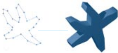
Extruded polygon cross section.
