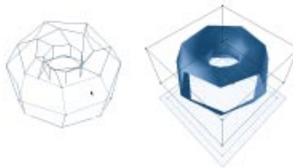
Emptying a polygon to create a hole in an object.
