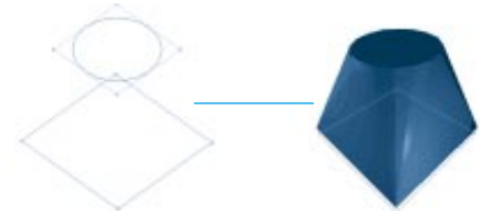
A Loft object is created by stretching a skin over a series of cross sections.
