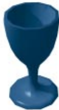
This object was created by rotating a lathe profile around a lathe axis.
